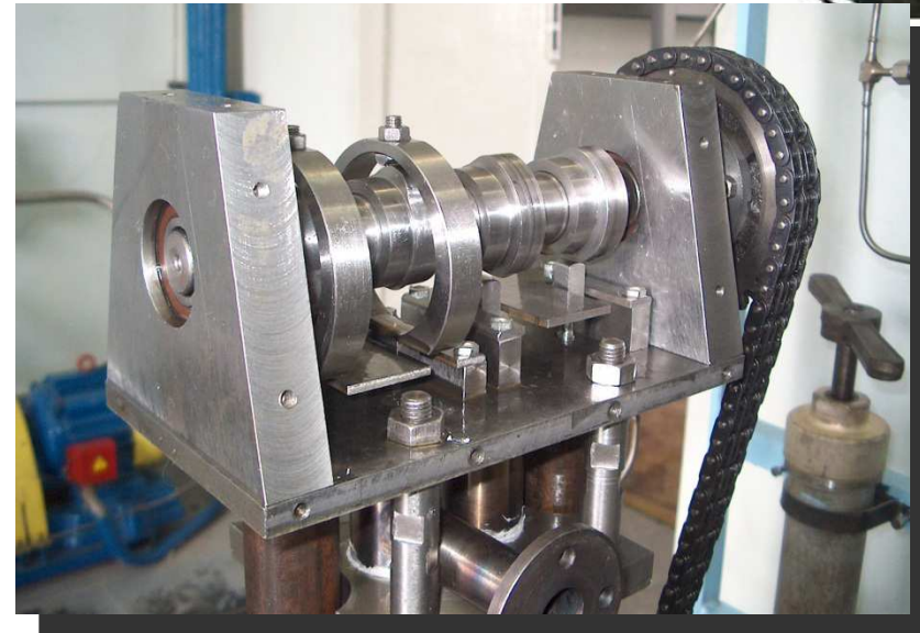
Gas-distributing mechanism. Cover is removed.
